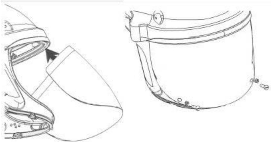
Ensure both securing screws and nuts are fitted.
